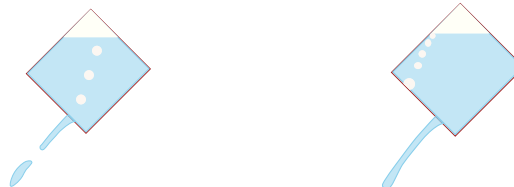
Fig. -9.11. Counter-current flow in a can (the left figure) has only one hole thus pulse flow and a flow with two holes (right picture).
